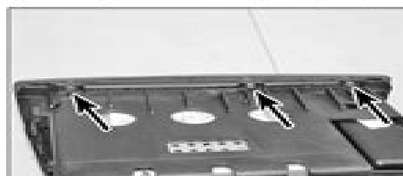
10.10a Undo the 3 Torx screws (arrowed) ...
