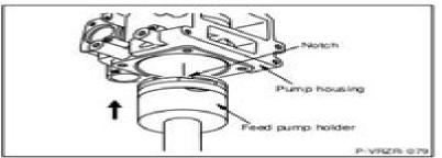
Position the feed pump assembly and the cover on the feed pump holder. Assemble the holder pins in the feed pump holes (2).
