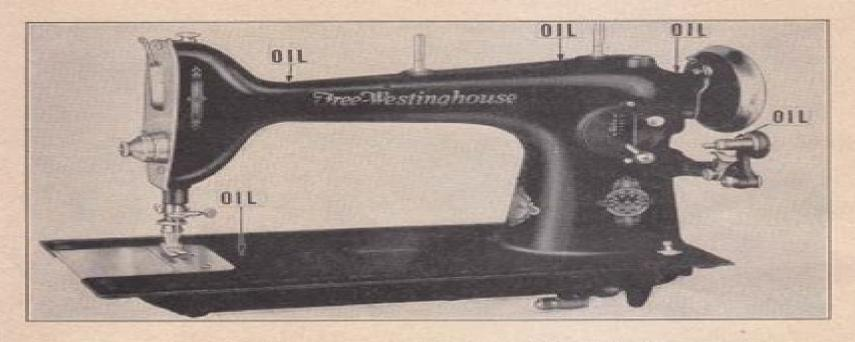
A sewing machine, like any other piece of fine machinery, needs oiling to insure smooth running and to prevent the wearing of parts. Use only the best oil, which you can get from us if your dealer cannot supply you. Poor oil will form a gum, causing the machine to run hard. Avoid oil which looks thick — good oil should be about the consistency of kerosene.
