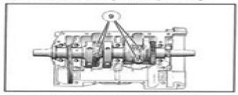
14. Torque connecting rod boits to specification (E).
