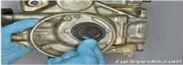
Inspect the crankshaft oil seal and replace it as needed.
