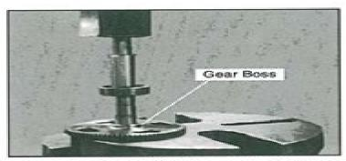
Apply Loctite<sup>™</sup> 609 to the pump shaft to help secure the bearing. Press on a new bearing.
