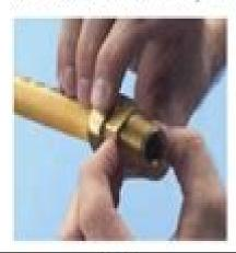
Step 4: Tighten with wrenches. Turn until nut contacts body.
