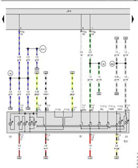
Light switch, Front and rear fog light switch, Onboard supply control unit, Light switch illumination bulb
