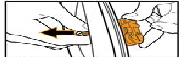
Step 2: Insert sensor into valve hole. *Ensure sensor close on the surface of wheel stop
