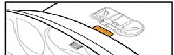
Step 4: Ensure the end of valve stem touched the rim
