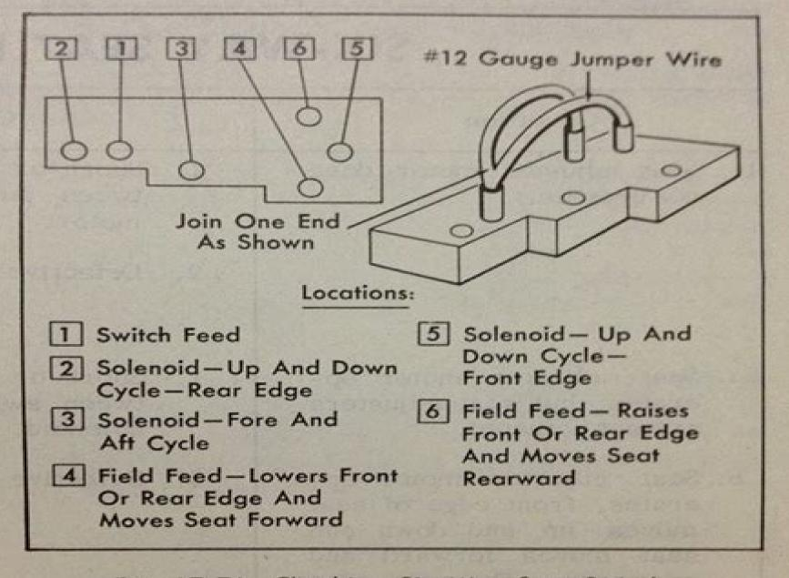
Fig. 17-76 Checking Six-Way Seat Switch
