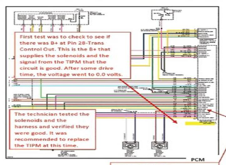
Key on B+ to TIPM was monitored at Pin 18. We were looking to see if the PCM was dropping B+. B+ remained when code set. We determined the PCM did not see a problem and turn off the relay.
