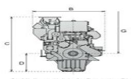
G : Minimum Height for Removing Piston
