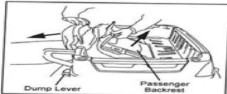
4. Lift the adjustment latch at the top of the passenger backrest. Raise the backrest to the desired position. Release the latch, making sure it locks into one of the three adjustment positions.
