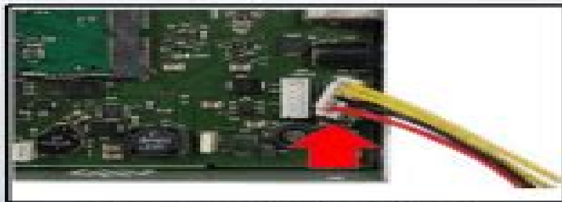
Figure 3: Removing the battery connector
