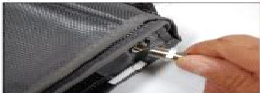
Figure 1: Unscrew the RF input connector
