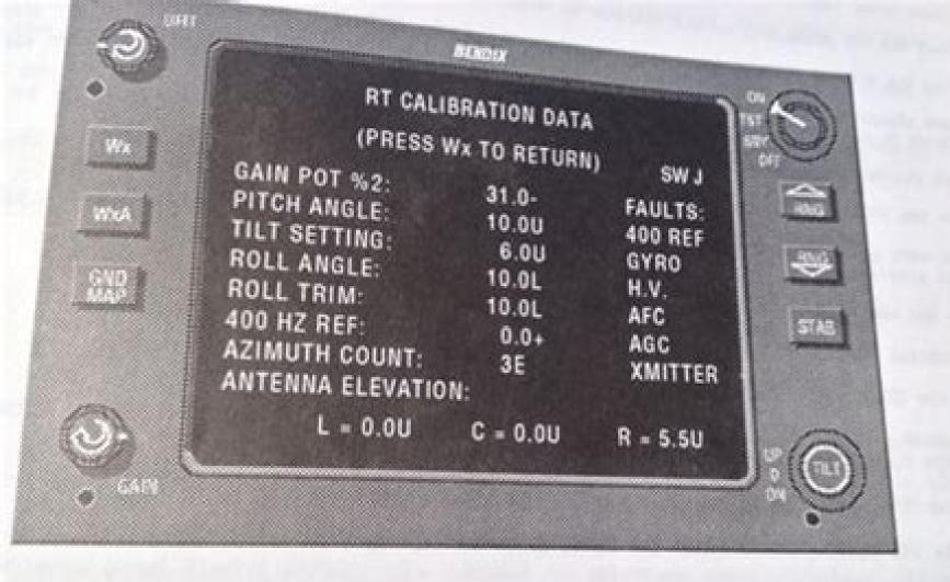
FIGURE 2-7 HIDDEN PAGE FORMAT FOR R/T CALIBRATION DATA
