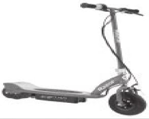
A NOTE: The unit must be traveling at least 3 mph (5 km/h) before motor will engage. Kick start to at least 3 mph (5 km/h) while applying the throttle to engage motor.
