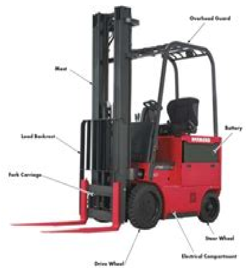
Figure 7-1 Main Components
