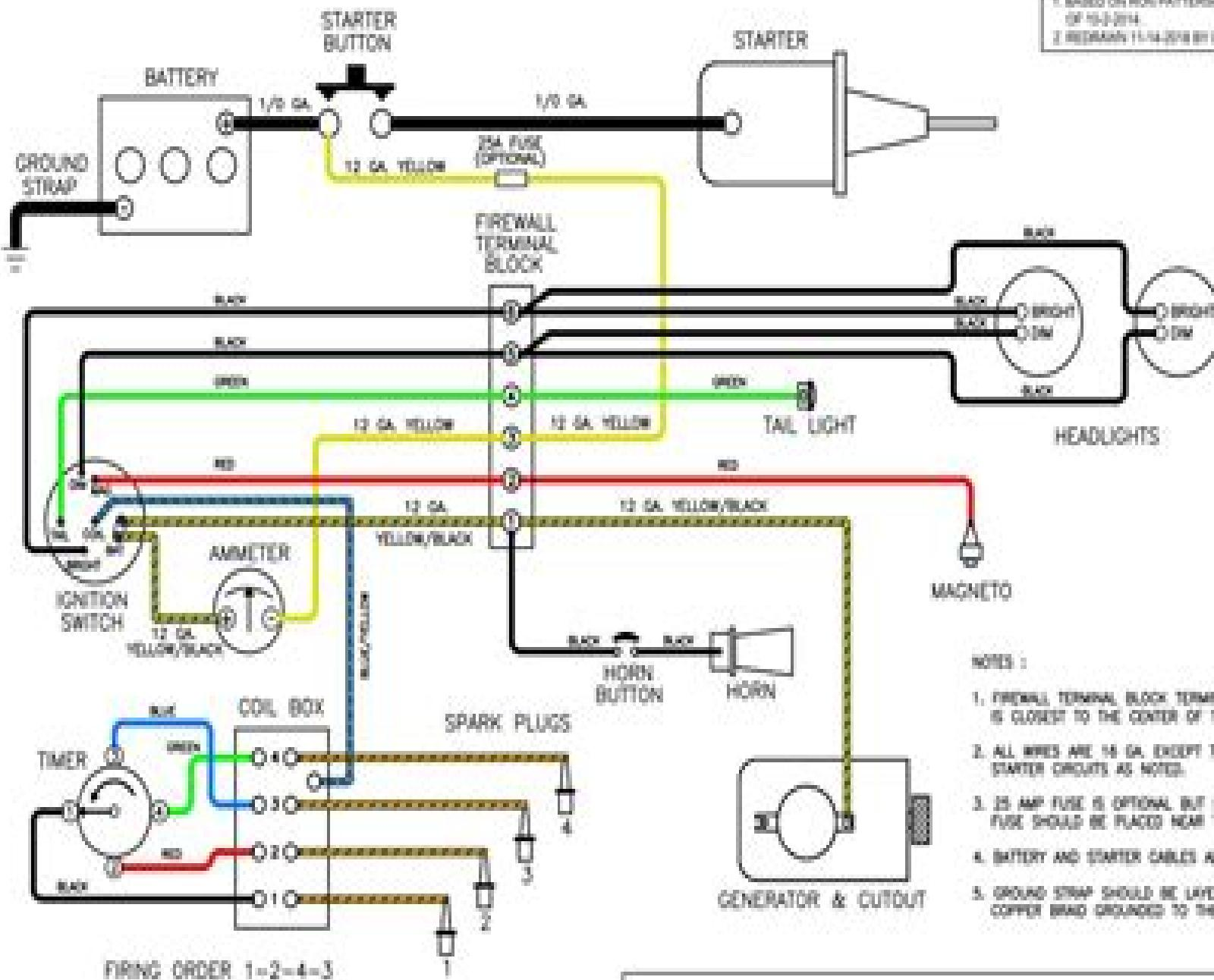
1919-1927 MODEL T WIRING SCHEMATIC
