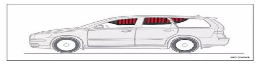
This system consists of inflatable curtains located along the sides of the roof liners, stretching from the center of both front side windows to the rear edge of the rear side door windows. It is designed to help protect the heads of the occupants of the front seats and the occupant of the outboard rear seating positions in certain side impact collisions.
