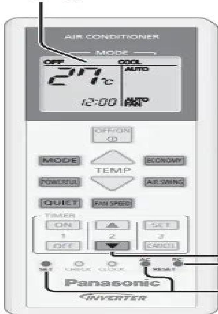
Press and hold for approximately 10 seconds to show temperature setting in °C or °F.
