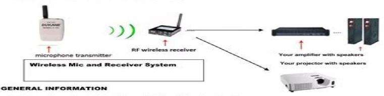
Thank you for purchasing the Dukane Wireless Microphone System WMIC1. This system operates using digital voice coding which is transmitted by radio frequency signal at 2.4GHz.
