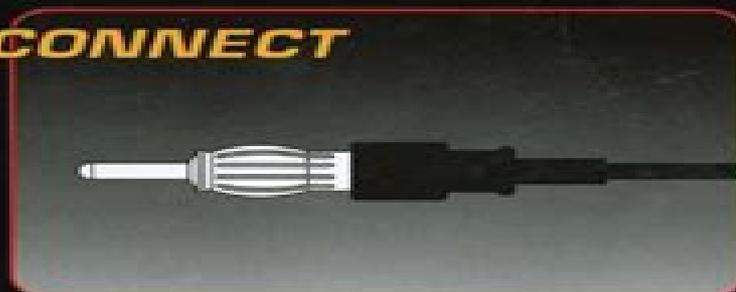
Plug the new antenna into the radio's antenna socket.
