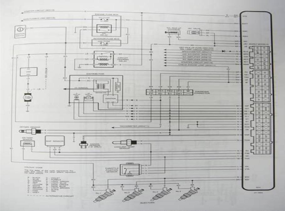
Fuel and engine management system circuit diagram, All models.
