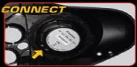
Install speaker using screws supplied with speaker and reattach speaker wires. Be sure to use proper polarity when connecting speaker. Test and reassemble fairing.
