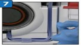
Place the larger blue tubing in the groove to the left and the smaller tubing to the right, close and latch the door
