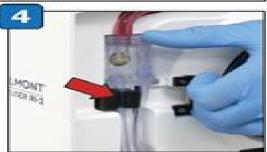
Place the pressure chamber into the pressure chamber well and press the infuse line into the air detector
