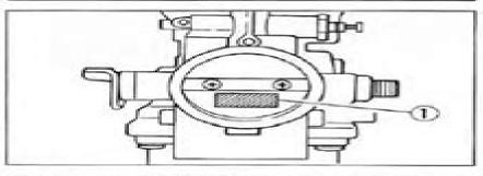
Hitch one end of spring to the boss ① and turn the other end ② clockwise by one turn and hitch it to the cable guide properly.
