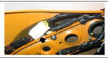
Voltage regulator - Remove the front central cover to reach it.
