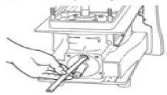
IMPORTANT: The correct clearance is .025 inch (0.64 mm).
