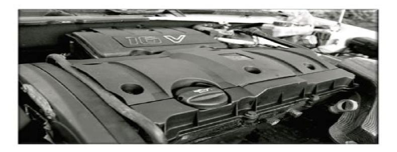
The TU5 has a displacement of 1587 cc, with a bore of 78.5 mm and a stroke of 82 mm. It was initially available in 8- and 16-valve configuration, but only the DOHC 16V option remains. Power is 109 PS (80 kW) in most current applications, the same as the DV61.6 L Diesel engine, although a sporty 122 PS (90 kW) version is used to power the Citroën C2 VTS. The TU5 has been used in motorsports by both Citroën and Peugeot.
