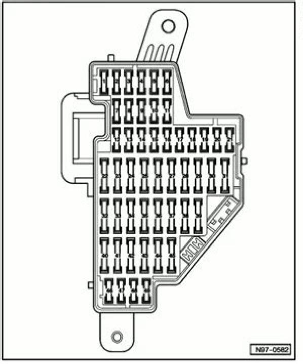
Fuse arrangements "SC" on fuse panel, in instrument panel, left
