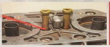
TOP, before liefts and after. While it is cleamer on the outside, it's the big improvements on the inside that really matter. ABOVE, we used this rebuild kit from Badke Services, which includes critical components such as needle valve, float, accelerafor pump disphragm, and idle richness screws, LEFT, if your early has been sitting outside, add a few drops of Liquid Wrench to threaded areas to help make them satisfies to cermowe.
