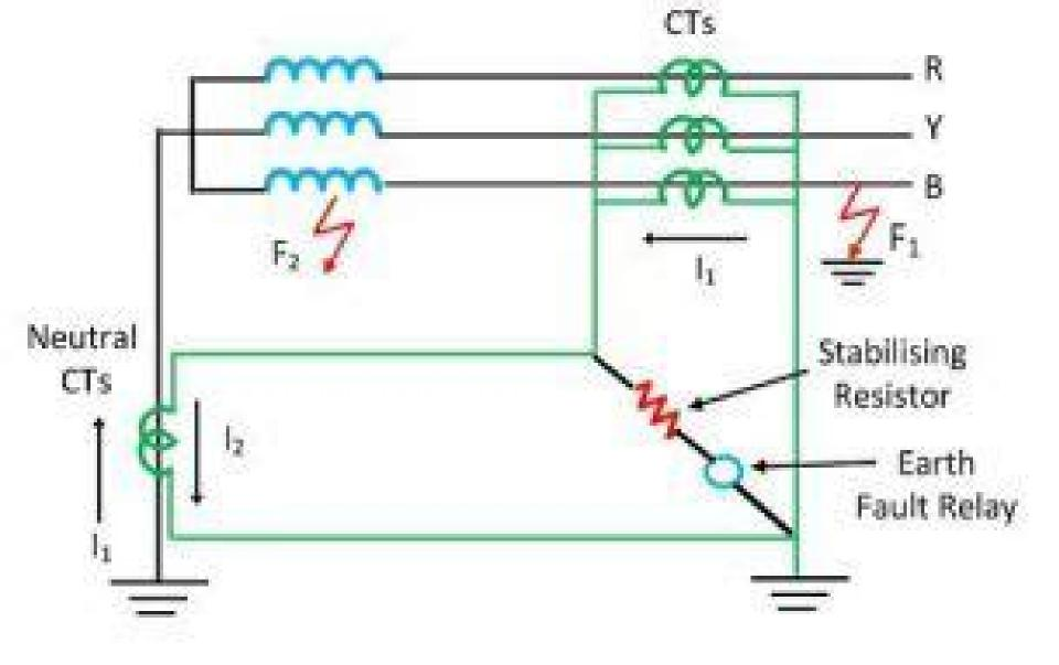
Restricted Earth Fault Protection Connected Earth Fault Relay
