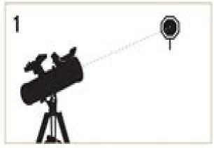
The finder is one of the most important parts of your telescope. It helps you locate objects and center them in the eyepiece. The first time you assemble your telescope, you need to align the finder to the telescope's main optics. It's best to do this during the day".
