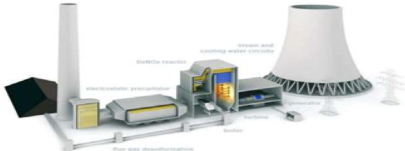
VIRTUAL VIEW OF THERMAL POWER PLANT
