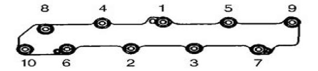
Fig. 6: Installing Exhaust Manifold Cylinder Head Retaining Nuts Courtesy of GENERAL MOTORS CORP.
