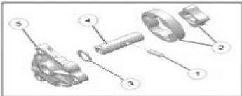
Grasp the complete oil pump assembly by the drive shaft(i) and install the assembly into the crankcase.
