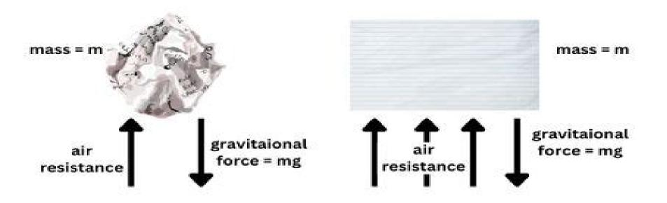
Paper with same mass will have same gravitational force applied. But, the air resistance on sheet of paper is greater than the air resistance on the crumbled paper.
