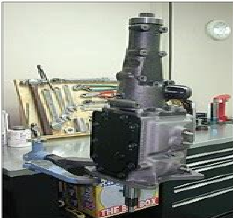
The Toploader is bolted to the holding fixture with two bolts on the passenger's side of the transmission. This allows work to be done with the Toploader in either the horizontal or vertical position. Between the holding fixture and the workbench, the 100-plus-pound transmission requires a stable platform. (Photo Courtesy David Randa)
