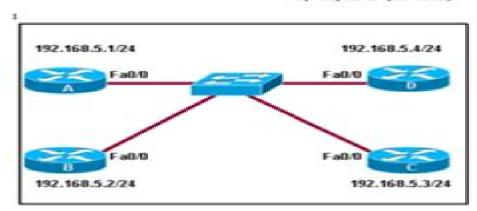
Refer to the exhibit. Routers A. B. C. and D are all running OSPF with default router IDs and OSPF interface priorities. Loopback interfaces are not configured and all interfaces are operational. Router D is the DR and router C is the BDR.
