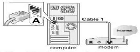
Step 2: Disconnect the Ethernet cable from the computer
